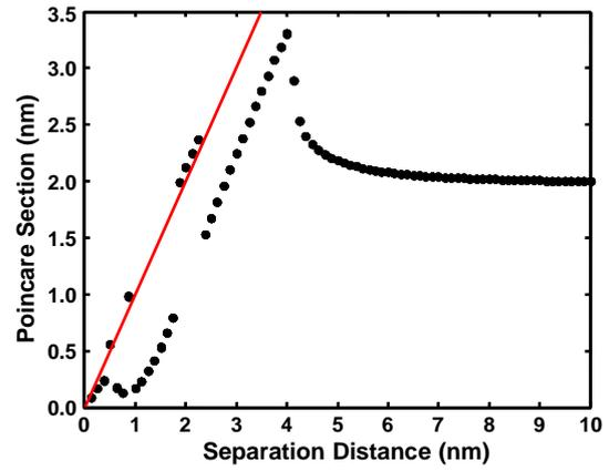
Figure 2. Simulated bifurcation diagram of the dynamic responses to excitation near the fundamental frequency. The separation distance is the control parameter.
