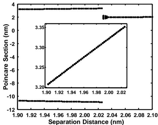
Figure 6. Simulated bifurcation diagram of the dynamic response to excitation near two and a half times the fundamental frequency. The insert contains an enlarged plot of the upper branch for the smaller separation distance values. The separation distance is the control parameter.
