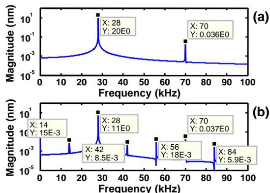
Figure 9. Spectral plots of simulated AFM response to dual frequency excitation for (a) inactive conditions and (b) active conditions.
