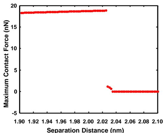
Figure 8. Maximum tip-sample interact force values for the separation distance ranges and response conditions presented in the bifurcation diagrams for (a) excitation at the fundamental frequency and (b) excitation at two and a half times the fundamental frequency.
