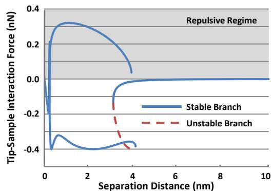
Figure 7. Maximum tip-sample interaction force values calculated from the results of the AUTO analysis that were used to produce the bifurcation diagram.
