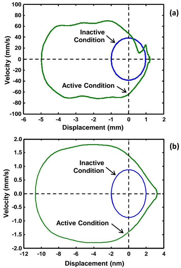
Figure 4. Simulated phase portraits of dynamic responses to excitation near two and a half times the fundamental frequency for (a) a macro-scale test apparatus and (b) a micro-scale AFM cantilever probe.
