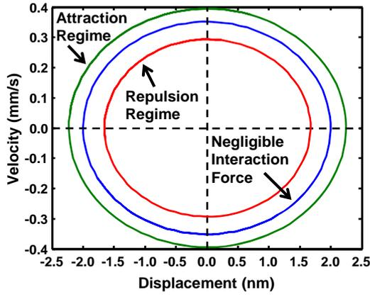
Figure 1. Simulated phase portraits of dynamic responses to excitation near the fundamental frequency for three different separation distances.
