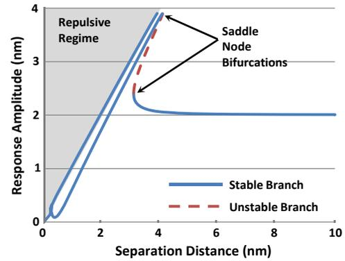
Figure 3. Bifurcation diagram produced using AUTO bifurcation and continuation software for excitation near the fundamental frequency. The separation distance is the control parameter.
