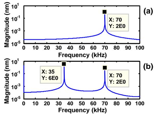
Figure 5. Frequency spectrum corresponding to dynamic responses of simulated AFM probe excited near two and a half times the fundamental frequency for (a) inactive conditions and (b) active conditions.
