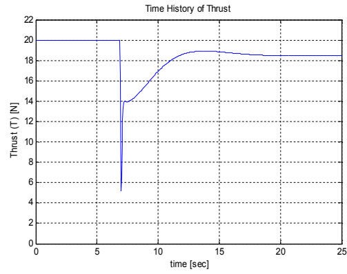
Figure 9. Thrust considering 20% uncertainty in the mass of the ducted fan
