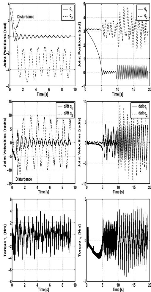
Fig. 3. Orbital stabilization of the Pendubot: left column for the orbital recovery under the randomly added quick disturbance, right column for the transfer from one orbit to another
