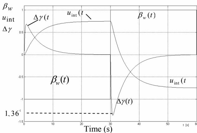
Fig. 4. Oscillograms for coordinates of control system motion for the integral autopilot structure
