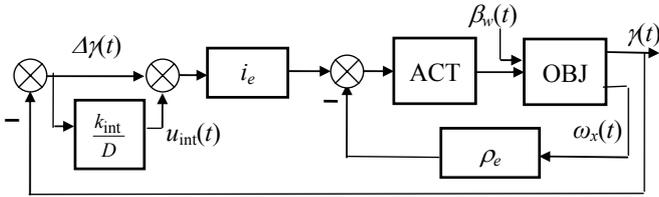
Fig. 3. Integral autopilot structure for the roll channel
