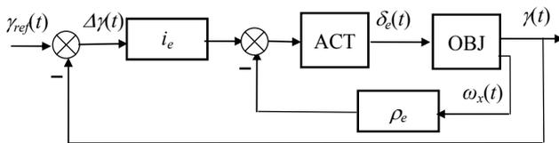
Fig.1. An integral autopilot structure for the angle of roll channel
