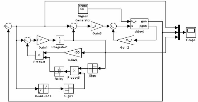
Fig. 6. Analog solution of the astatic control algorithm
