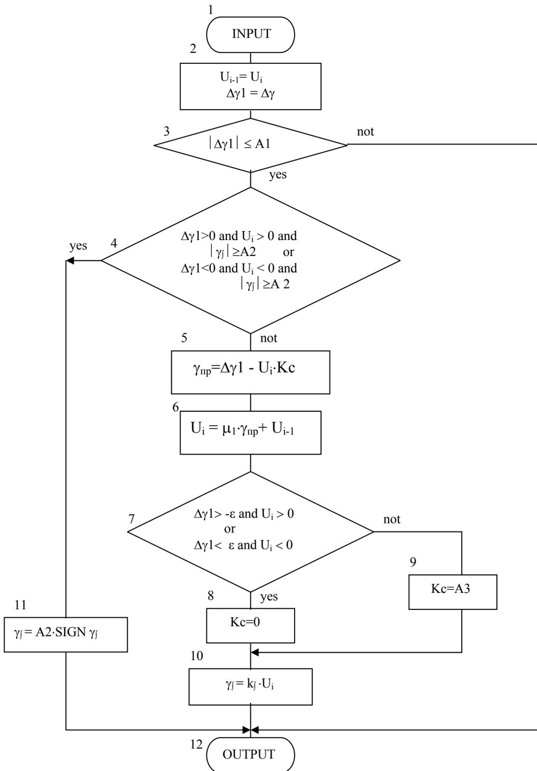
Fig. 8. Block-scheme for a possible digital realization of the astatic control algorithm
