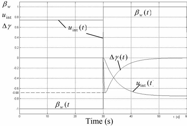
Fig. 5. Oscillograms for coordinates of control system motion in the integral autopilot structure with the ideal nullification
