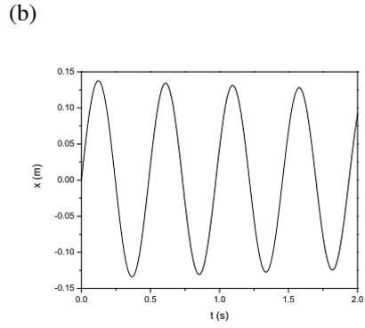
Figure 2. Displacement response obtained from multiple scales analysis, for (a) the first 20 seconds and (b) the first 2 seconds.
