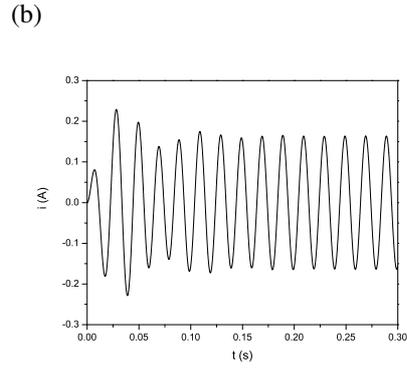
Figure 3. Current response obtained from numerical integration, for (a) the first second and (b) the first 0.3 seconds.
