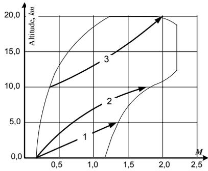
Some points have been chosen along all trajectories. Feedback coefficients in each point have been calculated by a modal method for thrust and trajectory channels.
