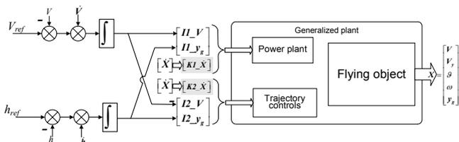
Fig.3. The structure of energy control system with modal correction
