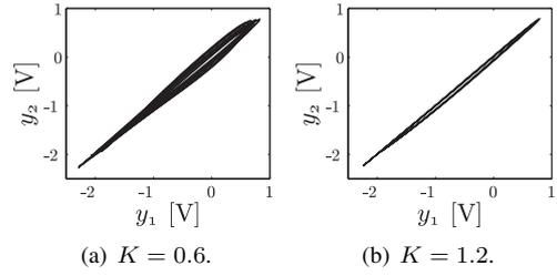
Figure 2. Synchronization of the two coupled systems.
