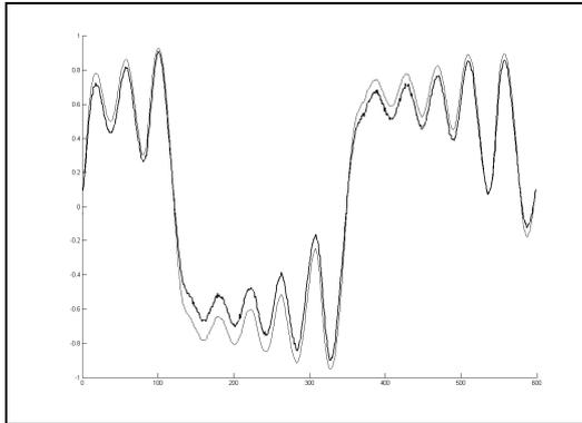
Figure 1 - Dynamics of the Chua's circuit (top). Measured values (solid line) and predicted values calculated by recurrent LS-SVM (thin line) - bottom.
