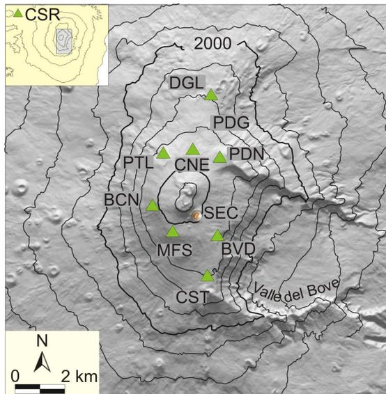
Figure 2. Magnetic monitoring network on Etna volcano.
