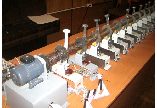
Figure 1. Multipendulum mechatronic set-up MMS IPME.
