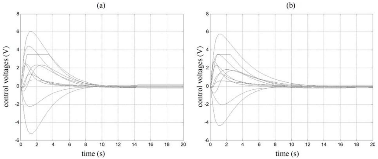
Figure 3. Control voltage signals  $u_1, \dots, u_{11}$  corresponding to a) initial controller and b) optimized controller.
