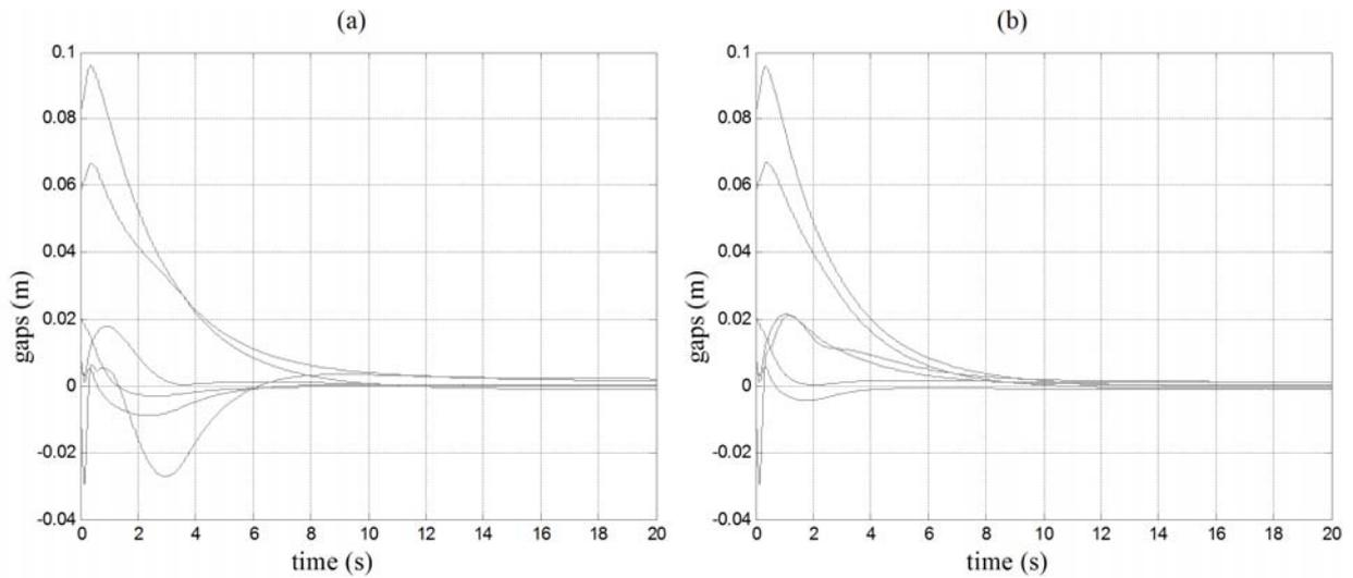
Figure 4. Transient processes of gaps  $g_1, \dots, g_6$  corresponding to a) initial controller and b) optimized controller.
