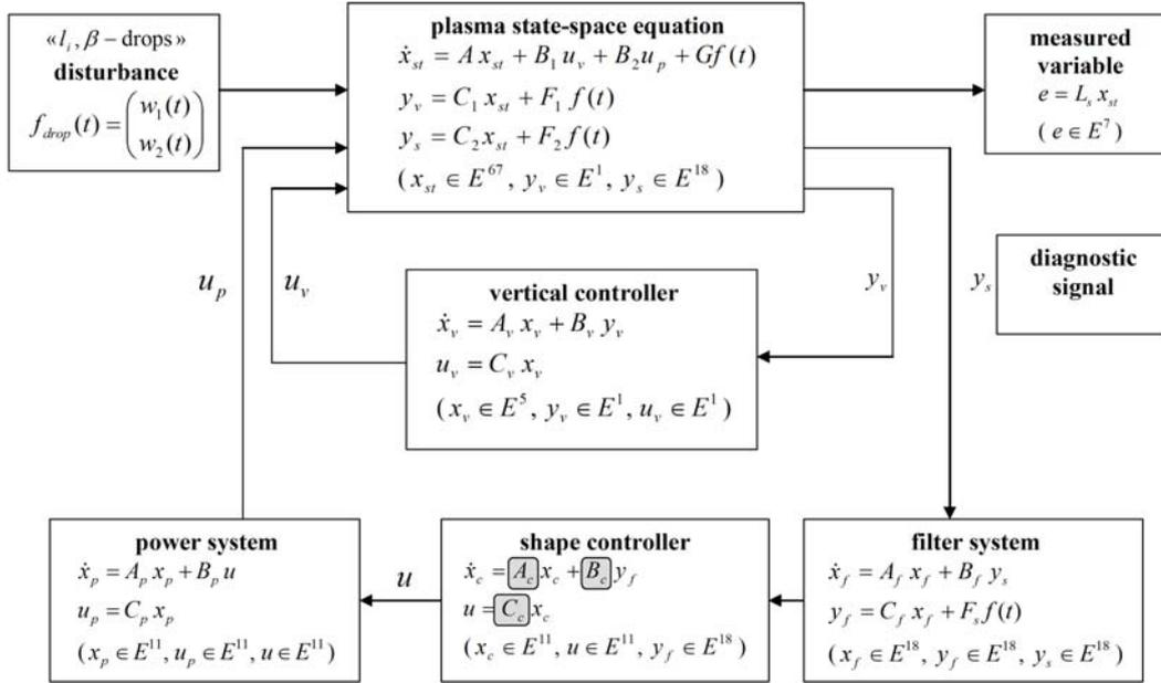
Figure 1. Structural model of ITER plasma control system.
