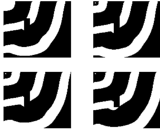
Figure 5: Propagation of autowaves from the source which are located at top-left corner on the network. The waves continue to propagate around the frozen cells on the array.
