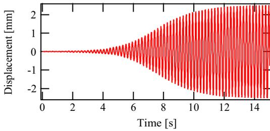
Figure 2. Time history of the displacement of the macrocantilever in the verification experiment
