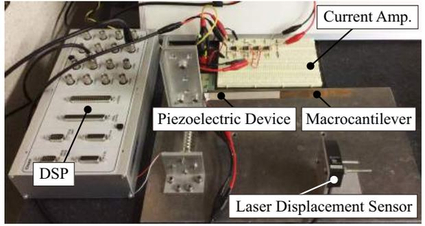
Figure 1. Picture of the experimental setup based on the theoretically proposed method
