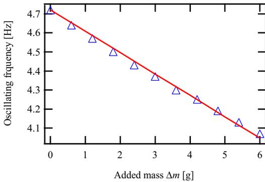
Figure 3. Relationship between the added mass and the oscillating frequency
