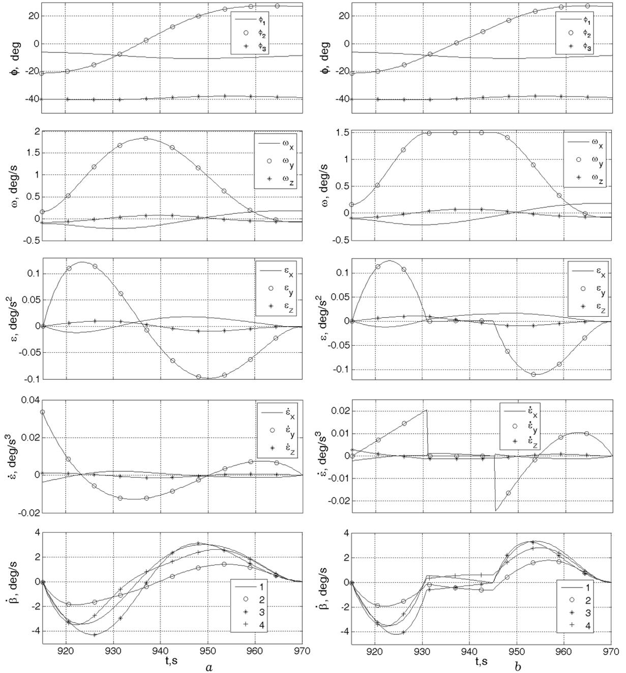
Fig. 3. Coordinates of the SC and the GMC at guidance by a rotation maneuver: *a* — without a limit of the SC angular rate in a *position transfer*; *b* — with such limit.
