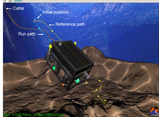
Figure 2. Path tracking of an underwater vehicle in the column and sea bottom.
