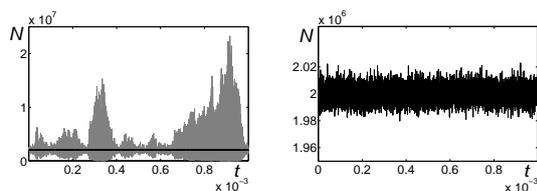
Figure 2. Time series of stochastic gas discharge system without control (grey) and with control (black) for  $\varepsilon = 2 \cdot 10^{-11}$ .
