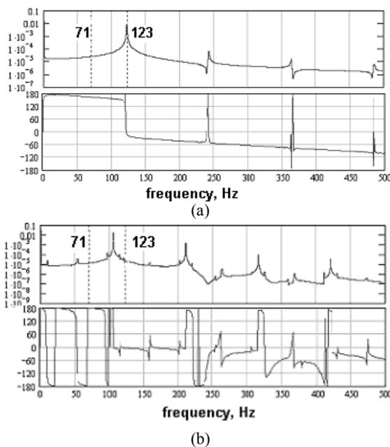
Figure 12. Bearing natural frequency shift due to wear: (a) Bearing wear - 0.2 mm (b) Bearing wear - 0.4 mm
