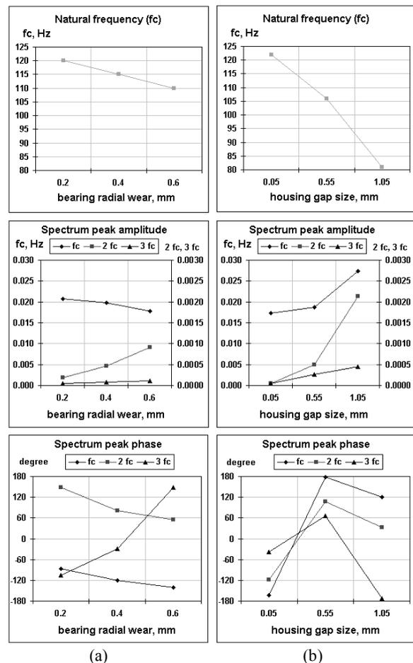
Figure 13. Diagnostics functions for bearing and bolting wear:
