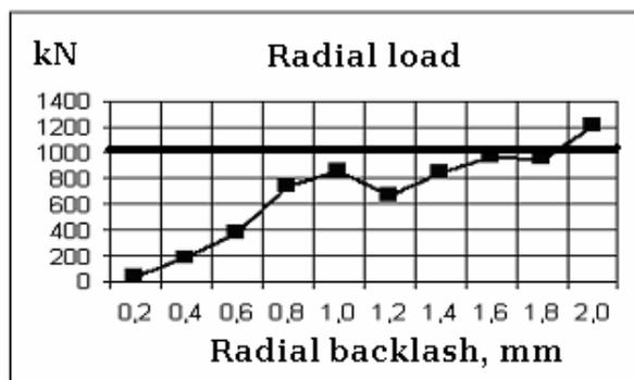
Figure 15. Radial load in the bearing by the wear.
