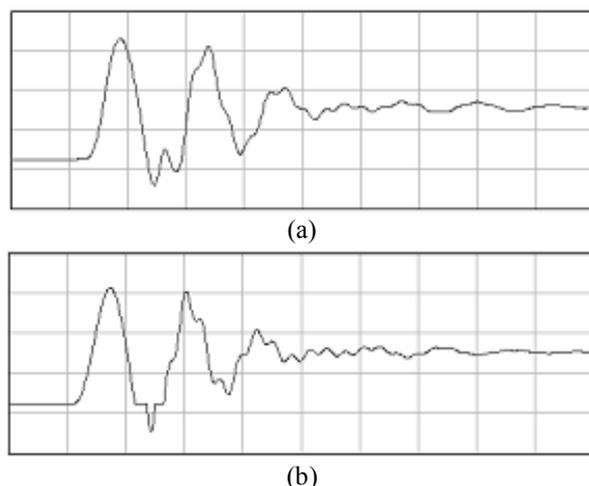
Figure 6. Nonlinear effects in the drive train: (a) Wear in the gearbox (b) Wear in the couplings
