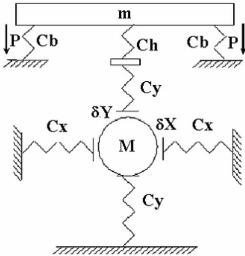
Figure 11. Calculation scheme of shaft, bearing and housing interaction.
