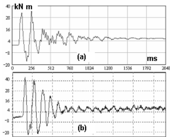
Figure 5. Nonlinear torsional vibration: (a) Calculation (T12) (b) Measurement
