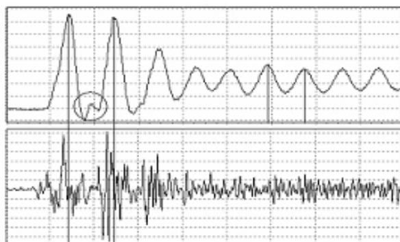
Figure 9. Non isochronisms in the Torque (upper) and Vibration (lower) signals due to wear.
