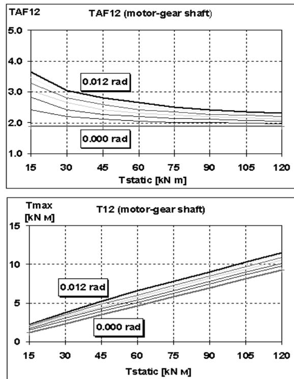
Figure 7. Nonlinear static torque influence: (a) TAF on motor-gear shaft (b) Peak torque  $T_{max}$
