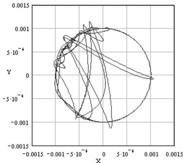
Figure 14. Calculation results of shaft center moving with the bearing and housing wear ( $\pm 0.001$  m).
