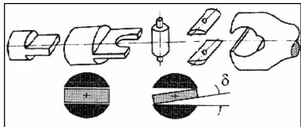
Figure 2. Spindle sliding block wear and backlash ( $\delta$ )
