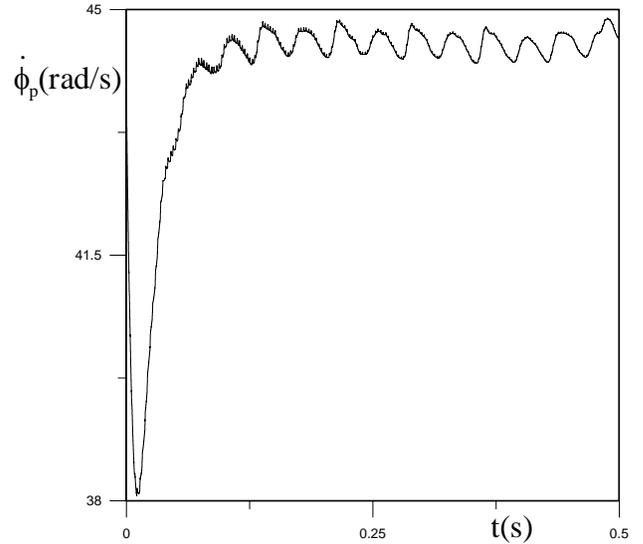
Figure 3: Time history of gear wheel velocity
