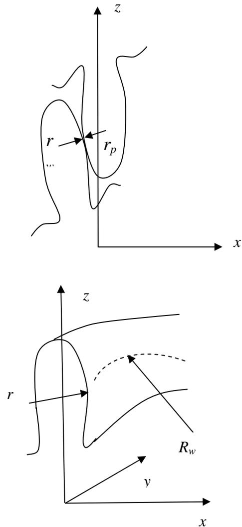
Figure 1: Principal radii of bodies in contact
