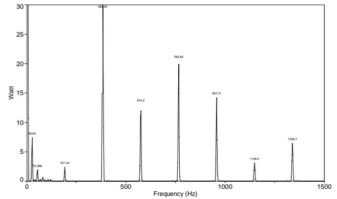
Figure 5: Typical spectral response of the impacting force of a gear teeth pair
